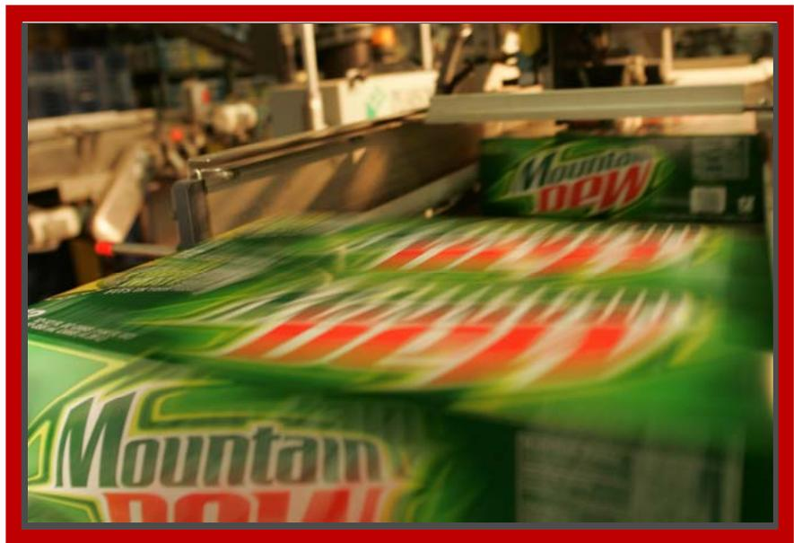
*Production lines typically run 120 hours each week. At the heart are Rockwell Automation control systems, which govern automated production from the unloading of empty cans and bottles to packaging.*
